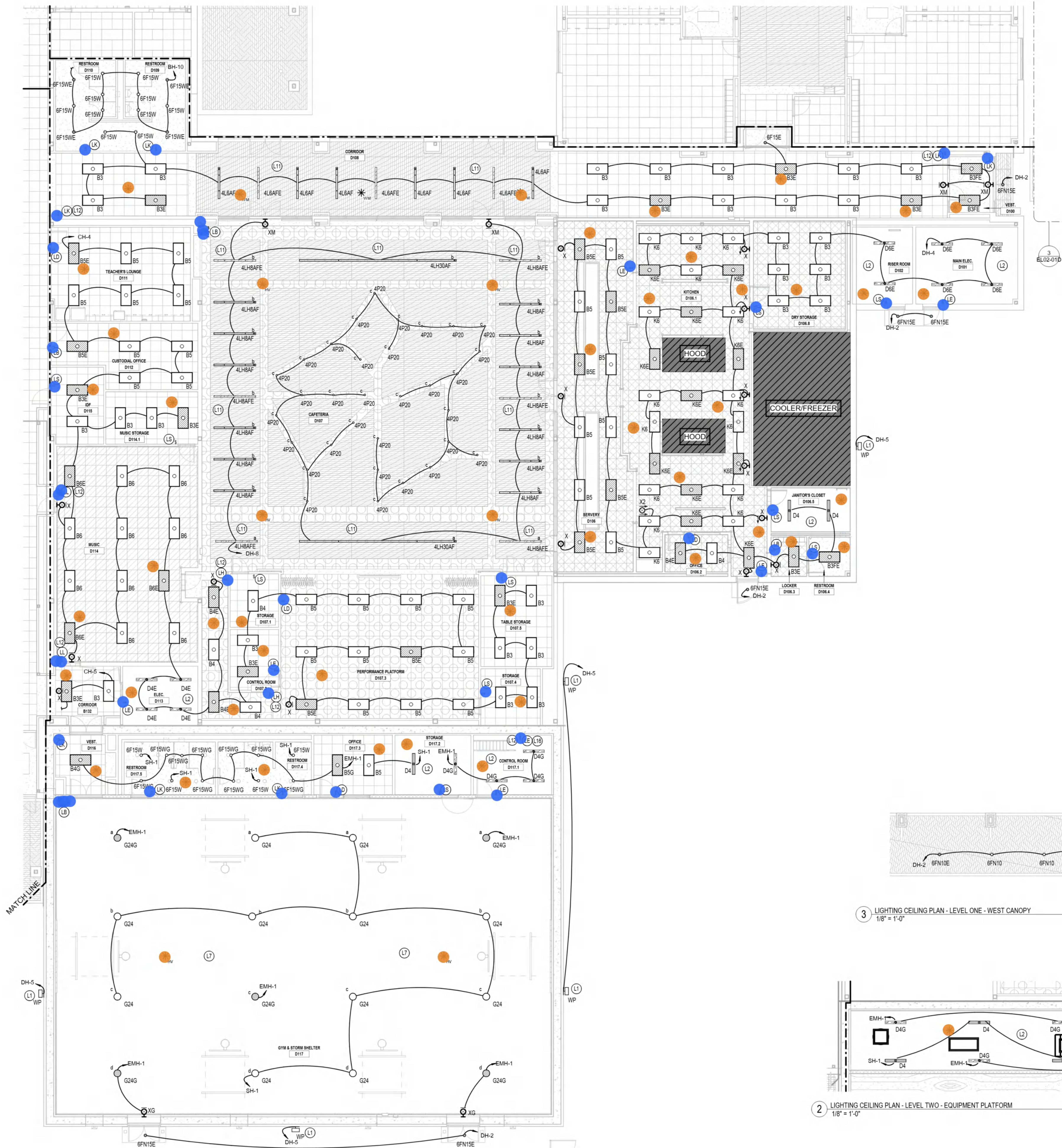
1 LIGHTING CEILING PLAN - LEVEL ONE - SEGMENT D 1/8" = 1'-0"
